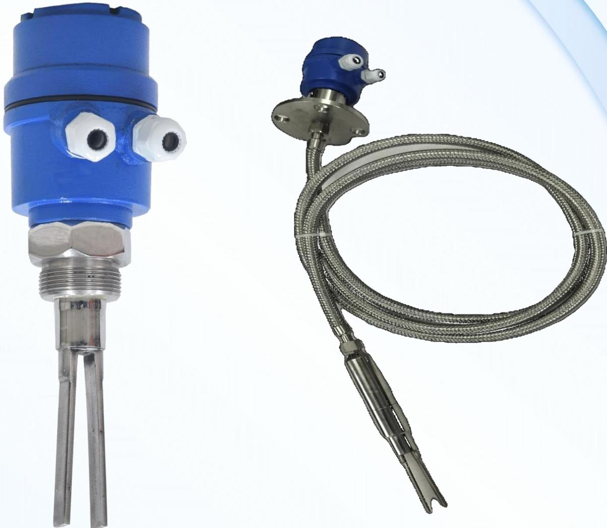
**VIBRATING FORK Level Switch** is specially designed for detecting maximum and minimum level in silo's filled with free-flowing solids, food grains, granules, powders etc. It can be used for detecting the level of material having overall size less than 15 mm. Variation of electrical parameters of the service material such as conductivity and dielectric constant do not affect its operation.
