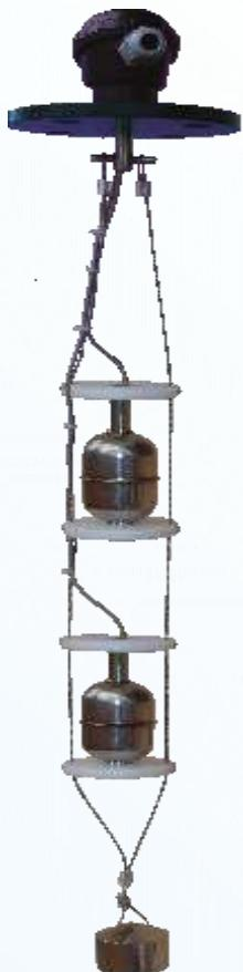
In Adjustable Float Level Switch mainly assembly is switch assembly which is provide signal with float movement & it is the fitted between two discs. These discs are easily adjustable on site & fixed with the help of grub screw as per required level points.
